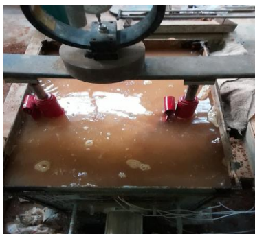
Figure 5. Saturated pullout box after the application of back water pressure
