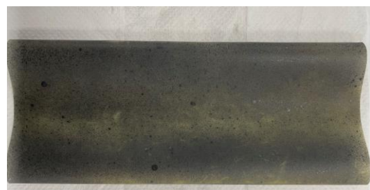
Figure 4: Speckle painted non-porous latex membrane
