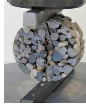
Figure 3. Tensile test: Failure along the grain surface and through the grains.
