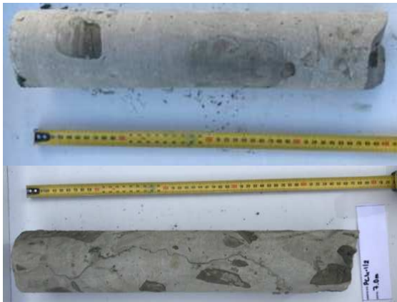
Figure 7 : Presence of inclusions (top picture) and joint between adjacent columns (bottom picture)
