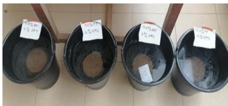
Figure 5. Wet curing of CBLS specimen in progress
