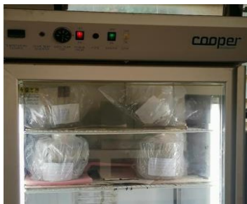
Figure 4. Moist curing of CBLS specimen in progress
