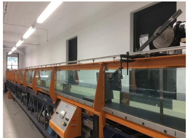
Figure 3. Tilting flume used for erosion testing.
