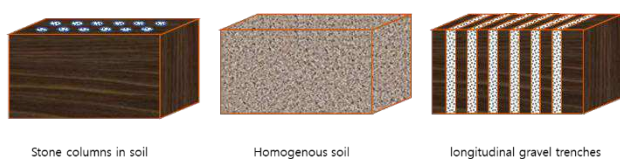
Figure 4. Modelling of stone columns in the soil.
