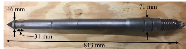
Figure 3. Tip screen configuration with dimensions.
