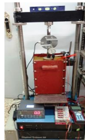
Figure 1. (a) Setup and details of the load-settlement test. (b) Soil container in the compression machine.
