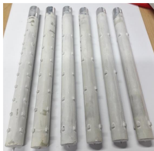
Figure 6. Model piles showing the different spacing between nodules (after Lalicata et al. , 2021).
