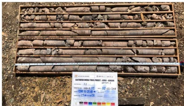
Figure 2. Rock core samples for PTP-V1-01; borehole 1DBH-A092.
