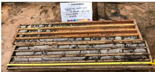
Figure 3. Rock core samples for PTP-V1-02; borehole V1-PTP2-BH2.
