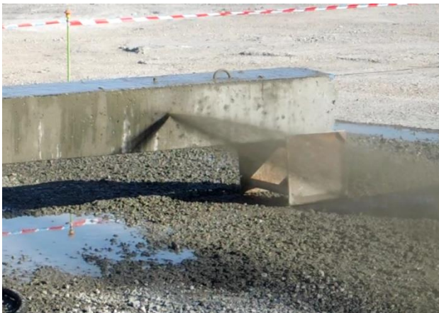
Figure 6. Shaft grouted driven concrete pile full-scale model. Grouting test
