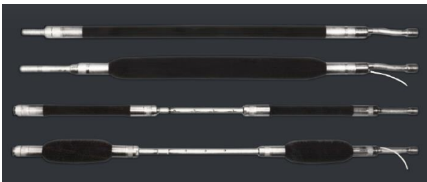
Figure 7. Single and double packer (courtesy of Petrometalic)
