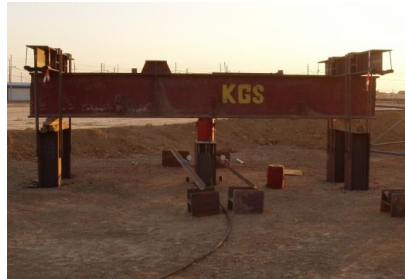
Figure 6. Static testing of the metal pile.
