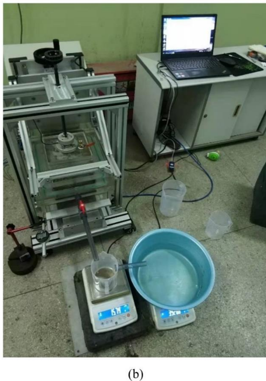
Figure 1. Shear-module-integrated seepage apparatus (a) schematic illustration and (b) photograph.
