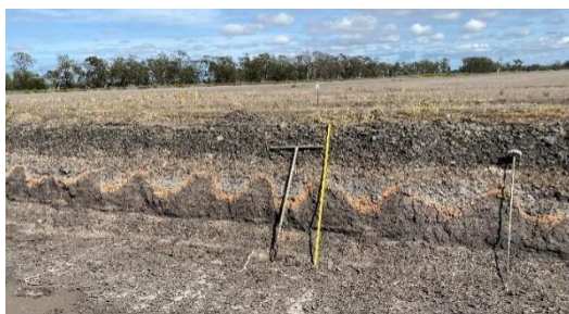
Figure 3. Photo showing typical plastic deformation of rail formation behavior during N2NS earthworks trial.
