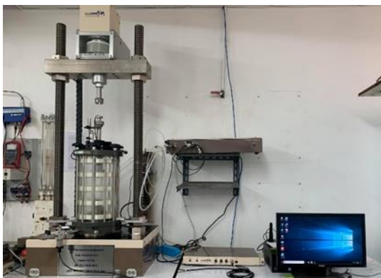
Figure 1. GDS Enterprise Level Dynamic Triaxial Testing System at the GTE Laboratory.
