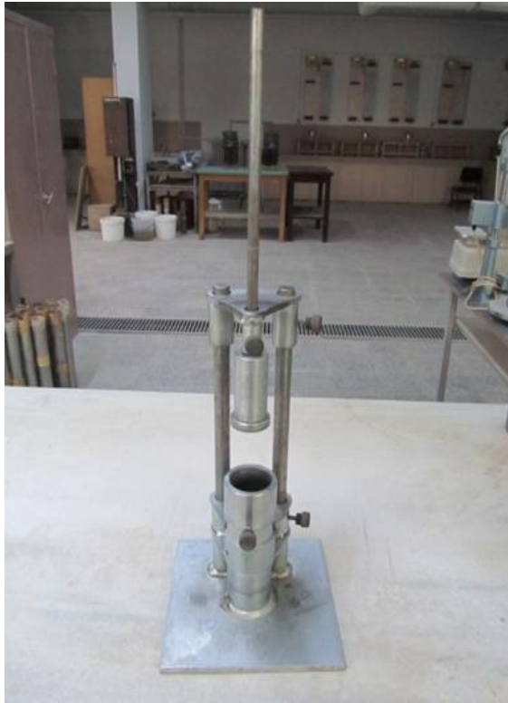
Figure 2. Modified Harvard compaction equipment used in the experimental program.
