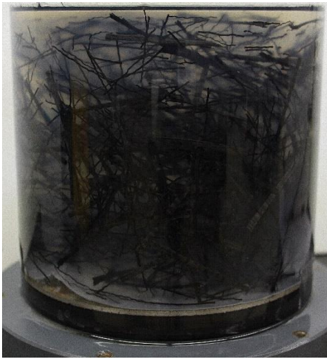
Figure 8: The fiber-reinforced transparent soil prepared as a part of this investigation.
