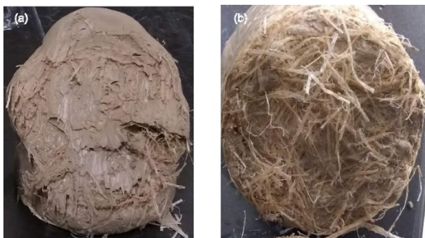
Figure 6. Samples of fiber-reinforced clay (2%-18 mm PP fibers) after failure (a) wet sample, (b) dry sample.
