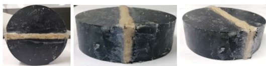
Figure 8. Top view and side views of the GCL specimens sandwiched between two PVC half cylinders and sealed with silicon paste (The images are from 30 mm height experiment)
