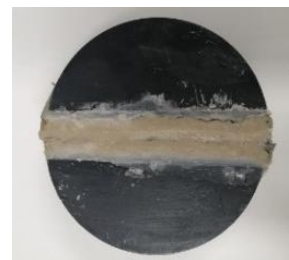
Figure 12. Top view of the two GCL layers sampled from the GCL overlap sealed in between two PVC half-cylinders (of 30 mm of height)
