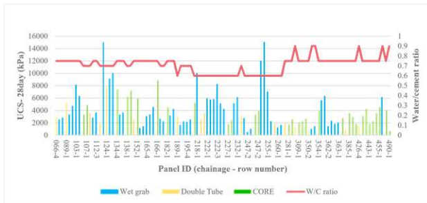
Figure 6. Unconfined Compressive Strength (UCS) versus Water/Cement Ratio (Djoric, A., et. al., 2021)
