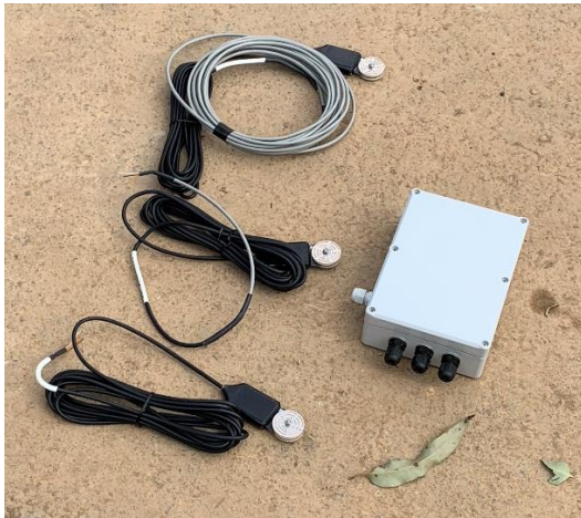
Figure 4. Closed DAQ with four ports for Teros 21 suction sensors
