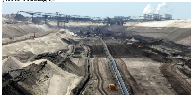
Figure 1. Conveyor bridge in an active open-cast mine in Lusatia.
