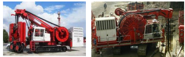
Figure 3. Bachy Soletanche HC05 piling rig
