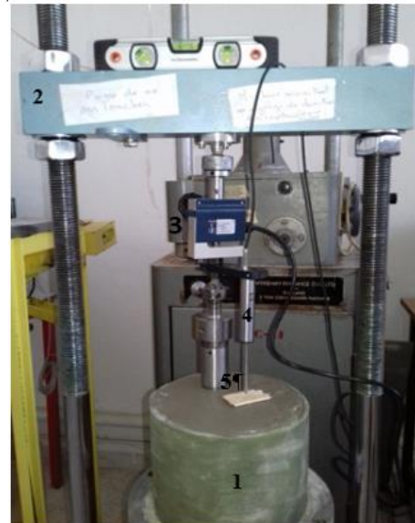
Figure 6 Complete mounting of the CST and measurement accessories of the triaxial load frame
