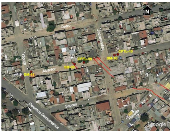
Figure 14. Location of borings, Colonia El Molino Tezonco site.
