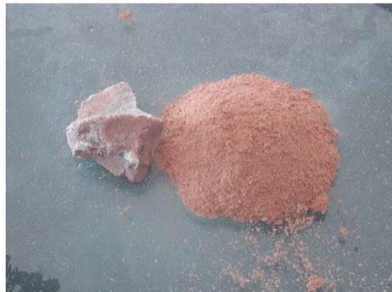
Figure 4. Comparison of Conglomerate (left) and siltstone after immersion of water (Margottini, 2004)
