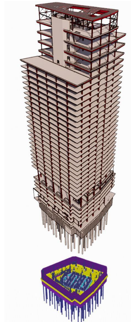
Figure 7. Soil-Structure Interaction combined 3D geotechnical and structural models.
