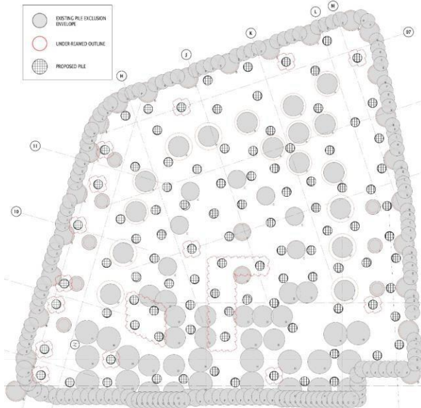
Figure 5. RIBA Stage 4 pile-enhanced raft layout of new piles on existing piles with exclusion zone.
