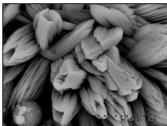
Figure 7. Zeolite crystalline structure in the modified mix, M4 (magnification = 9k)
