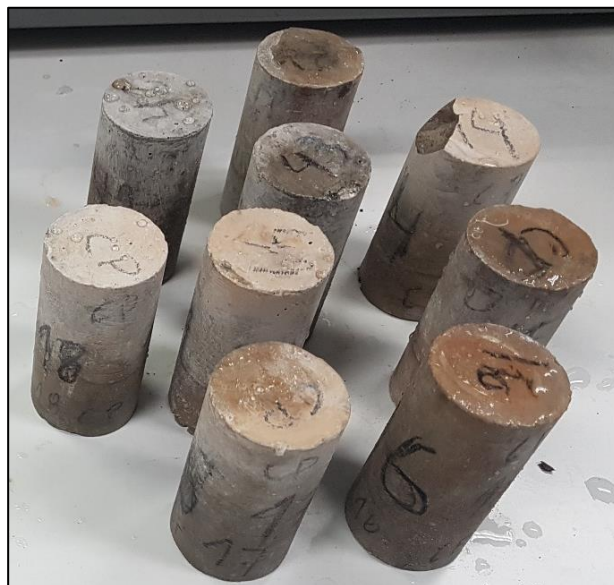
Figure 2. Samples after 30 days of supercritical carbonation at 20MPa and 90°C.
