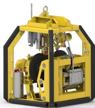
Figure 6. ROSON-ST seabed CPT system
