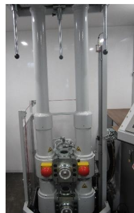
Figure 3. COSON 200 kN inside cabin CPT vehicle
