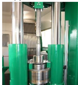
Figure 9. Twister, to connect the ST-rods
