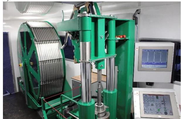
Figure 7. Folder, Sprocket, Twister, ST-rods and data transfer
