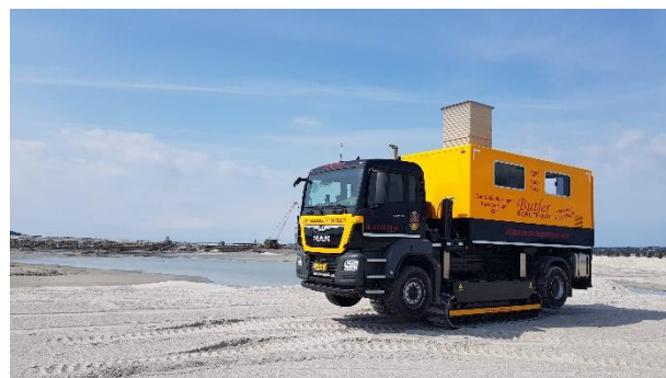
Figure 2. Track-Truck with HYSON 200 kN inside the cabin
