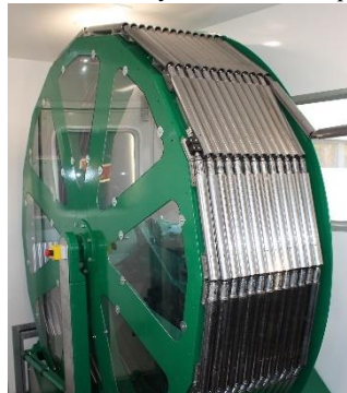
Figure 8. Folder, storage of the ST-rods
