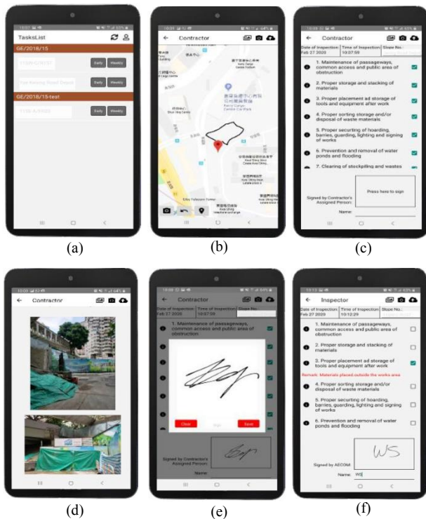
Figure 9. Mobile app for site cleanliness (a) dashboard; (b) site location; (c) checklist; (d) site photos; (e) contractor's signature; (f) comment by RSS.
