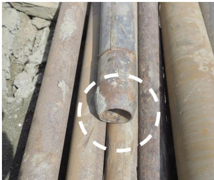
Figure 13. Example of poorly maintained device for geotechnical subsurface investigation (shoe of standard penetration device).
