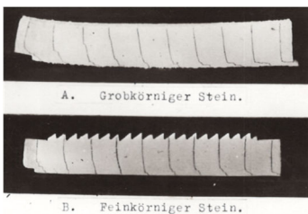
Figure 25. Influence of grain size with shear off just above the serration (Hvorslev, 1936).
