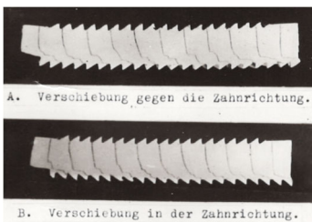
Figure 24. Influence of direction of serration (serration height 2.6 mm and spacing of serration 4.6 mm) with shear off just above the serration (Hvorslev, 1936).
