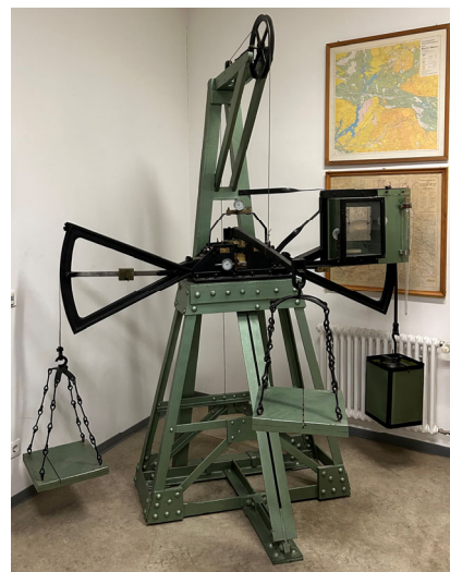
Figure 17. Krey shear test apparatus; original of the first fabricate at TU Berlin (© Adam, 2025).
