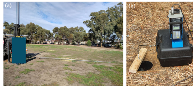
Figure 2. Set-up for NMM monitoring (a) access tube installation, (b) reading taken.
