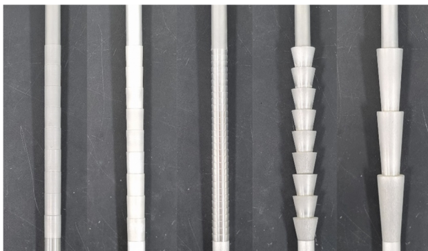
Figure 1. Geometry of textured piles used in this study. The parameter L represents the scale length and H is the scale height. The total length of the surface scale remains constant at 180 mm across all piles.
