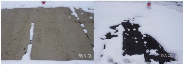
Figure 5. Performance of concrete-copper (B 1.2) and wide-spaced asphalt-plastic (A 1.2) HAPs during snowfall scenario
