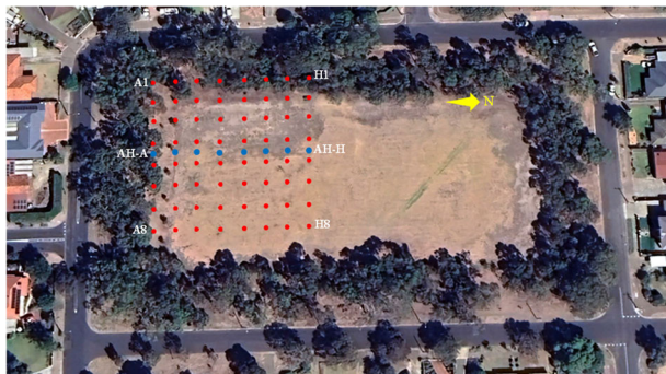
Figure 1. Surrounding of the study area (Google Earth Pro, 2024) showing access holes (AH) and ground movement monitoring points (A1 to A8).
