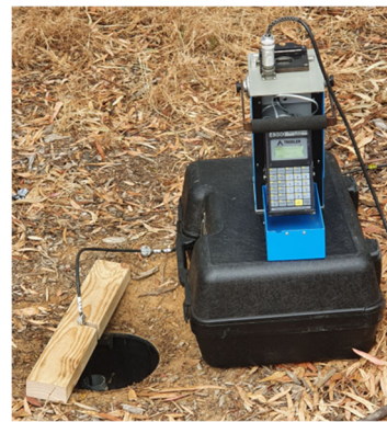
Figure 2. NMM with probe inserted in access hole to take reading.
