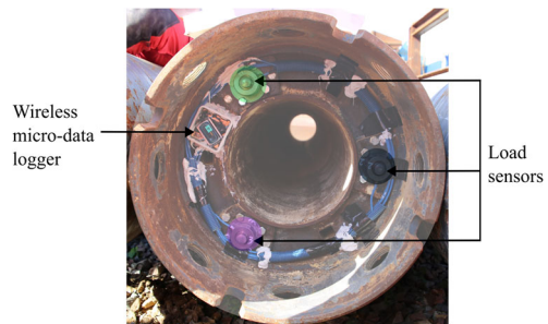
Figure 5. Instrumentation arrangement in hollow element, female extremity.
