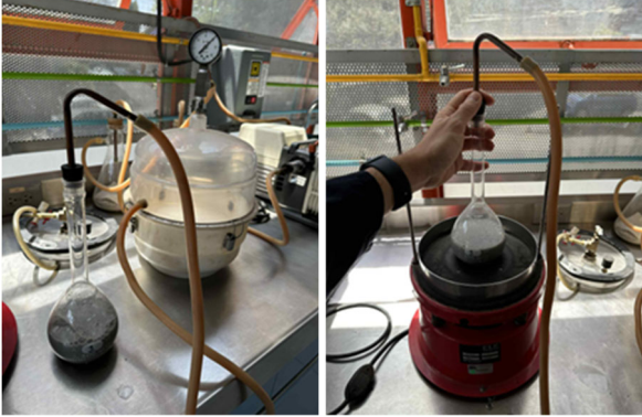
Figure 3. Test for determining the specific gravity of solid particles.
