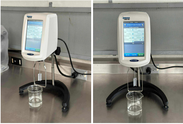
Figure 7. Rotational viscometer used in this study.
