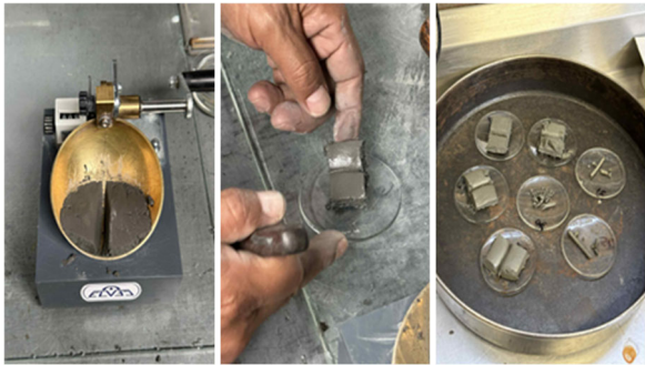
Figure 4. Test for determining the Atterberg limits.
