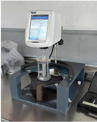
Figure 8. Test for obtaining the rheological properties of the tailings sample.
