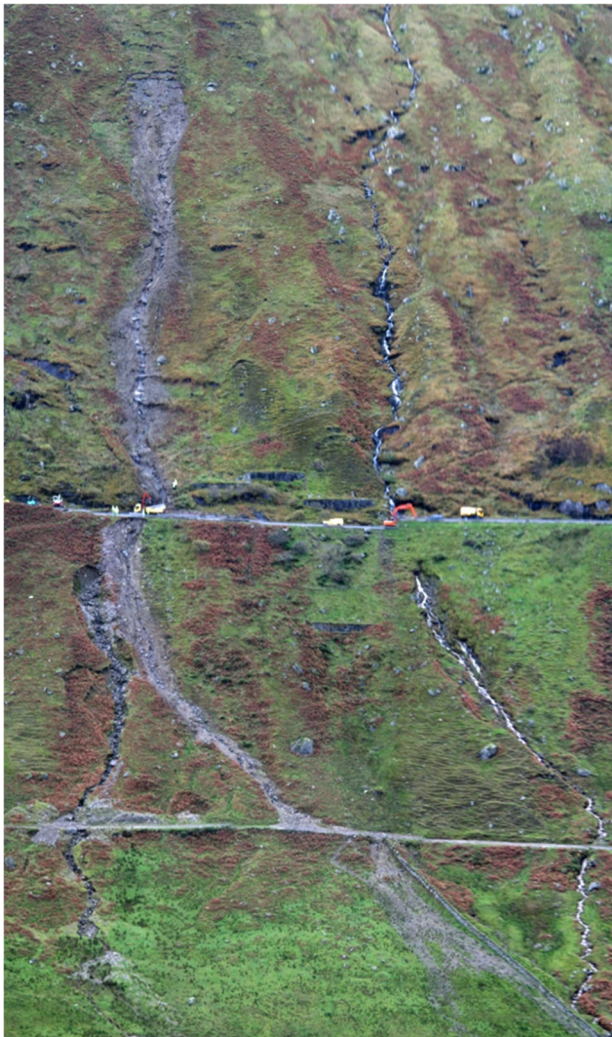
Figure 2. View of the debris flows above and below the A83 on the approach to the Rest and be Thankful. The head scar is at approximately 370 m Above Ordnance Datum (AOD), the A83 at 240 m AOD and the Old Military Road (OMR) at 180 m AOD.
