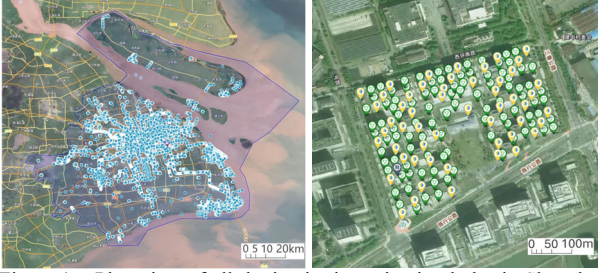
Figure 1. Plan view of all the in-situ investigation holes in Shanghai (left) used and CPT (green) - borehole (yellow) layout at a typical geotechnical investigation site (right).
