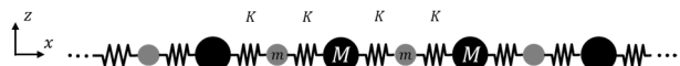
Figure 7. Example of a 1D lattice with two different masses ( M and m ) connected by identical springs.
