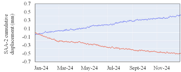
Figure 5. SAA-2 measured cumulative displacement.
