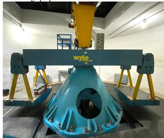
Figure 1. Geotechnical centrifuge at UENF.
