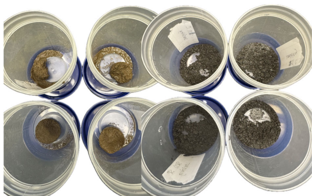
Figure 4. OS (left) and BS (right) after 18h submerged in DI water. The controls are shown on top and the MICP treated samples on bottom. The duplicate experiments are shown.
