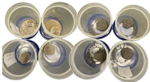
Figure 3. OS (left) and BS (right) after 3 weeks of curing. The controls are shown on top and the MICP treated samples on bottom. The duplicate experiments are shown.
