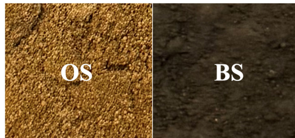
Figure 1. Slag materials OS (left) and BS (right).
