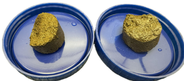
Figure 5. Treated OS after 18 h of slake test.
