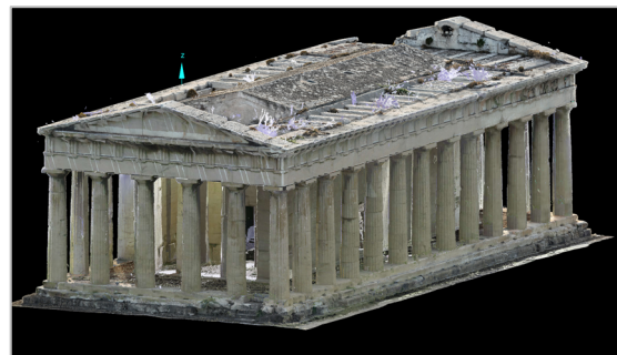
Figure 1. Hybrid LiDAR and SfM Point-Cloud model of the Hephaisteion and surrounding hillslope
