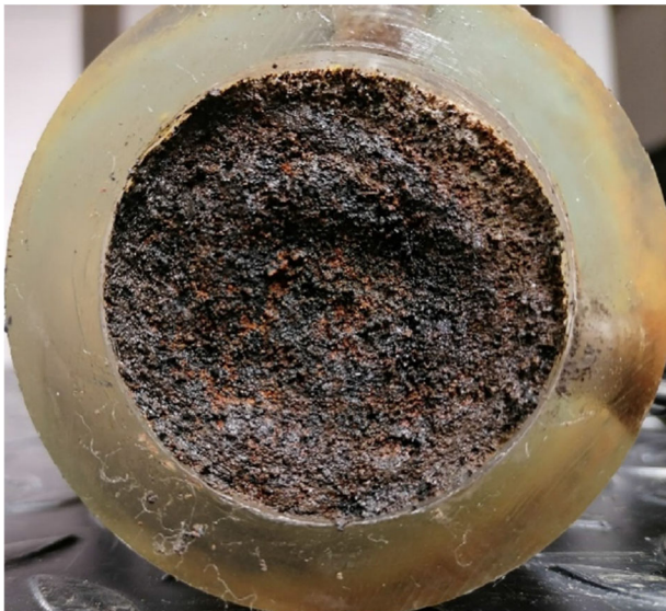
Figure 4. ZVI/lapillus mixture inside column A after disassembly.
