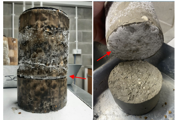
Figure 6. Ice lens formation in samples cured for 91 days after frost heave testing. The sample with 1% lime is on the left; 2% on the right. The ice lenses are highlighted by the red markers.
