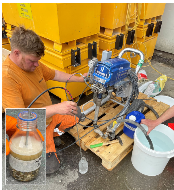
Figure 6 Injection test rig. Test with clear water. Insert shows a gravel filled bottle.
