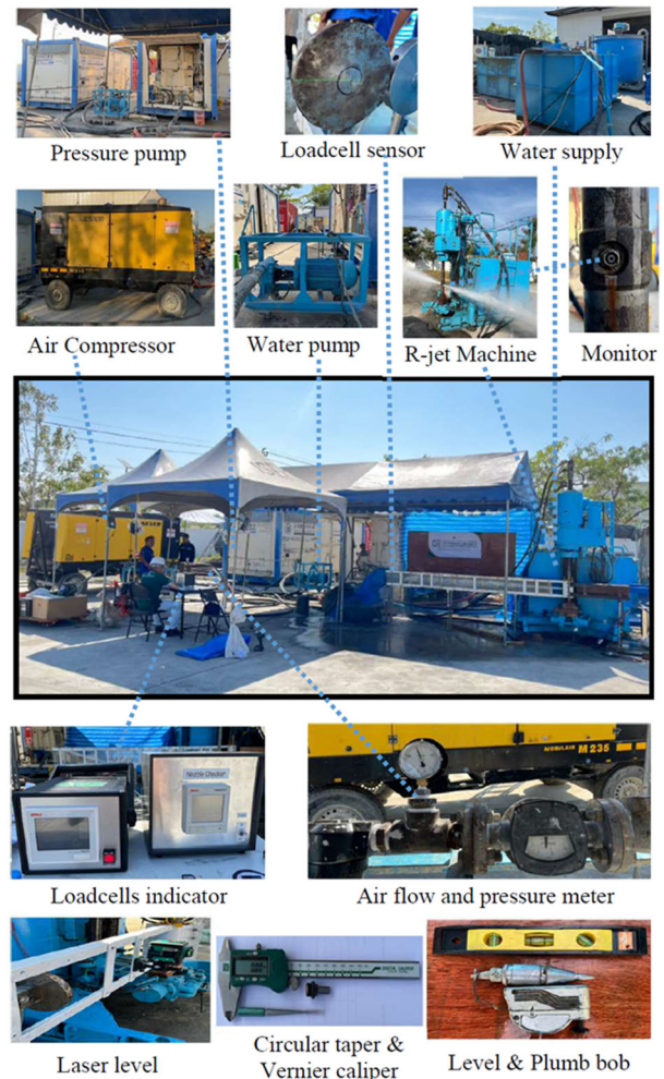
Figure 2. List of equipment and tools for the stream tests.
